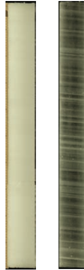
Figures 3a and 3b. (a) Top 53 meters of the GISP2 ice core firn (b) Annual layers of the GISP2 ice core at a depth of 1837 meters
