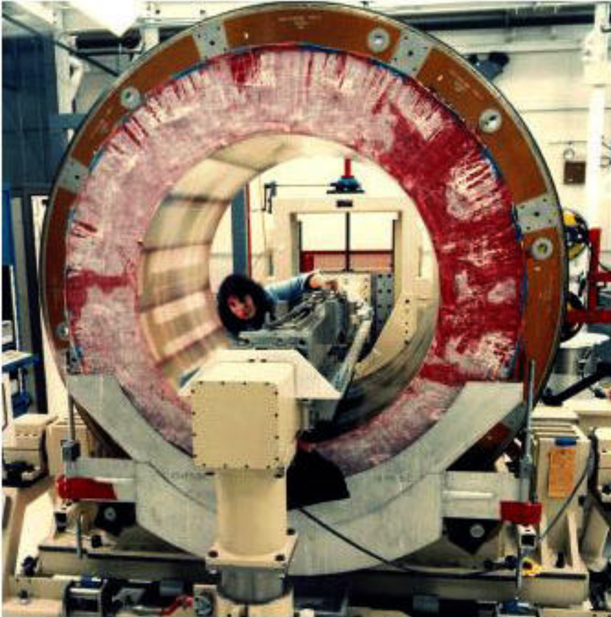
Polishing a CXO Mirror Shell
